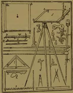
Fig. 14.-Pretonius's Plane-table.
